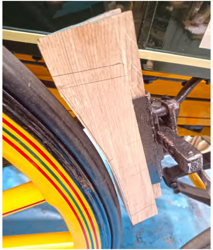
Fitting brake blocks. Alan Gaskell.
