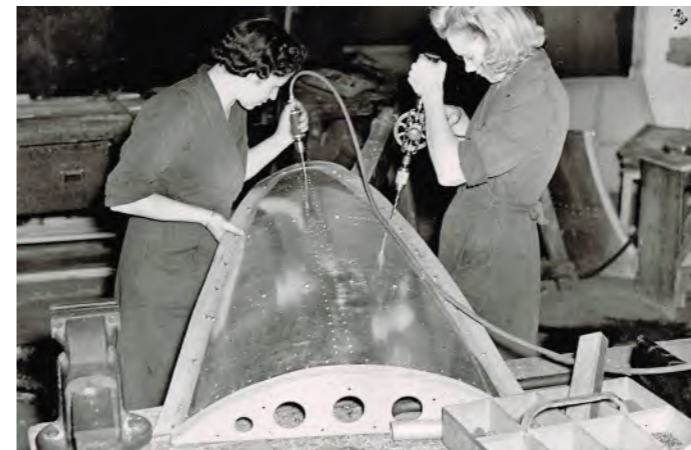
Two young ladies assemble a Halifax fairing, possibly the rear of an engine nacelle, using pneumatic and hand drills.
