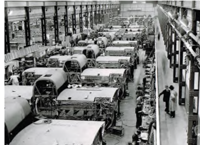
Above- Halifax production at Aldenham the assembly line for aircraft centre sections, with outer skins being applied.
