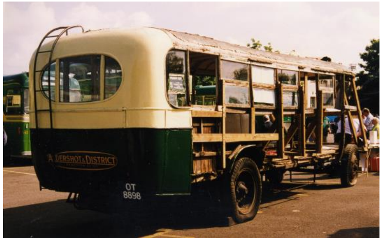
1928 Dennis E type bus under restoration
