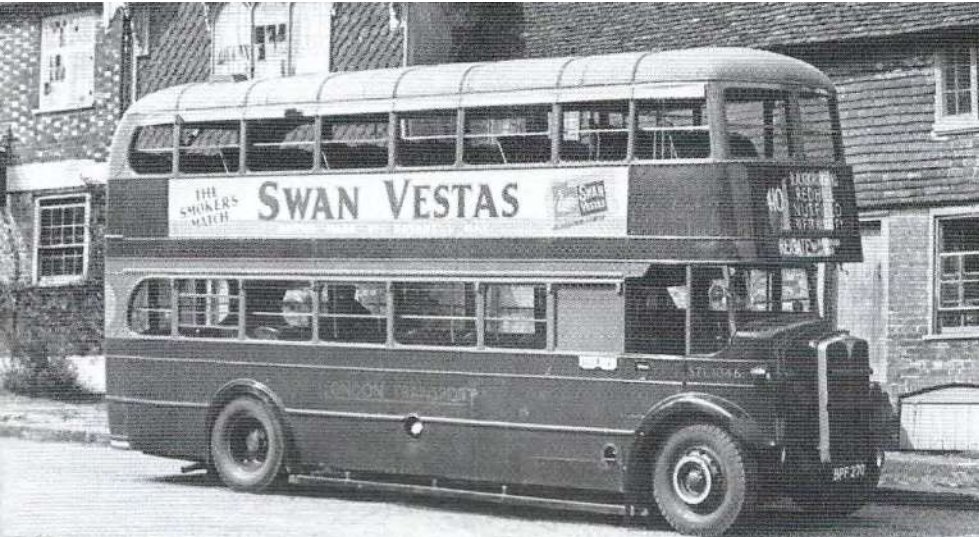
Unique were the twelve Godstone STLs, ordered by Reigate in 1933, but delivered to London Transport. These were essentially of provincial specification with their Weymann, lowbridge bodies, and made the 410 route from Bromley to Reigate their own until well into post-war days. STL1046 pauses at Godstone on a westbound journey. (Collection)
