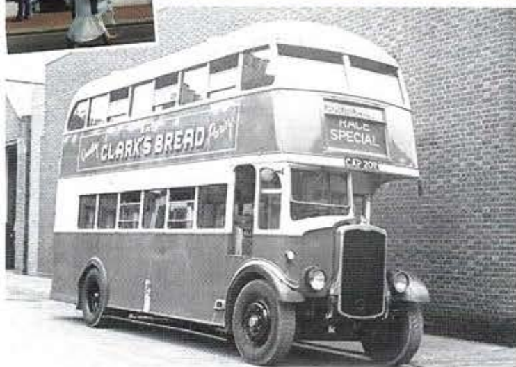
A Brighton, Hove and District ECW bodied Bristol COG5 about to set off for the racecourse in 1938. (Collection)
