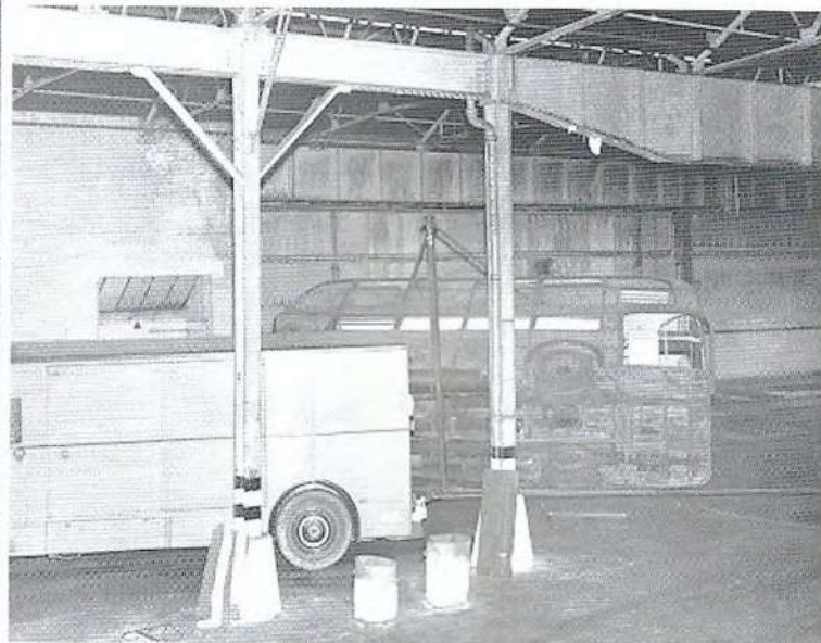
London bus RT106 was adopted as a training vehicle for LT staff and renumbered 1036TV. It is seen here at Hammersmith Trolleybus Garage in 1967 with shear-legs recovery equipment in place to demonstrate recovery of the vehicle into a vertical position. That equipment was transported in LT emergency lorries similar to that in the foreground. The bus's interior lighting had presumably been activated for photographic effect. (LT photo 67/182)
