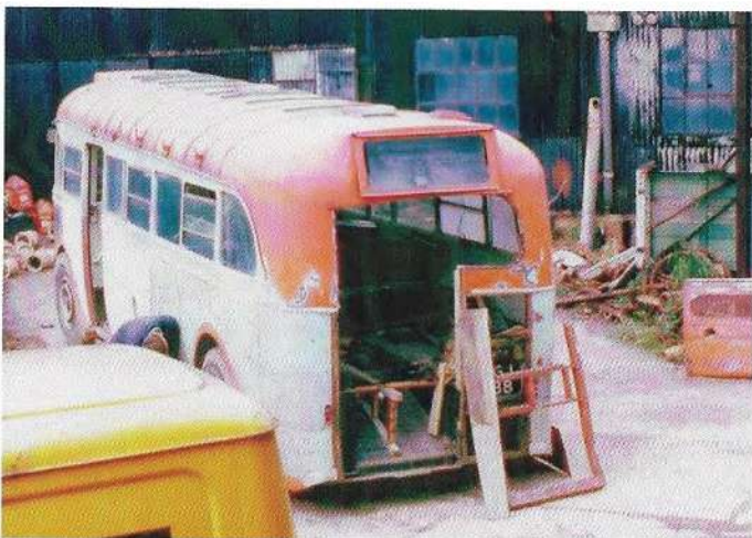
Probably during a lunch break - part of the rear framing made by Cottrell senior stands ready. The internal part of the wheelchair ramp added by the Sutton Coldfield people can also be seen. (Michael Wickham)
