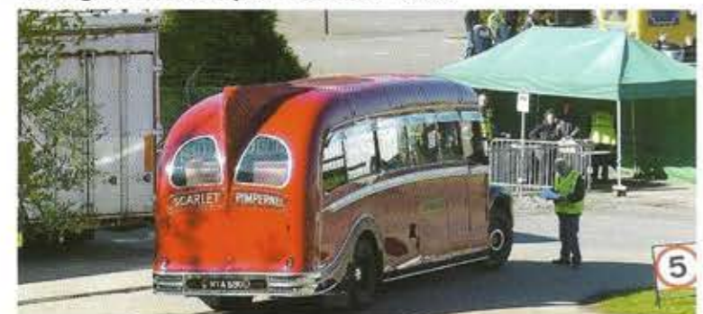
a rear view of Leyland Comet MYA590 displaying the distinctive Harrington tail fin.
