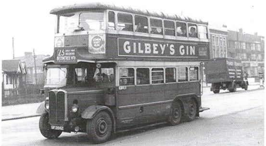
The AEC Renown six-wheel chassis was utilised by LGOC for their 'LT' class. One of those is seen here in East London post WWII. (Photo from the Edward Shepherd collection of the London Bus Museum)
