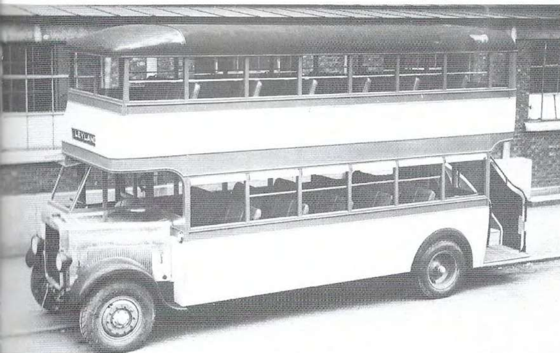
Leyland works photo taken in March 1927 of the prototype Titan. Note the unfinished bonnet which had just been altered to accommodate a new design of radiator grille from that originally fitted. In cross-section the Leyland low-height body matched the profile shown on a U.S Patent filed by Rackham while working for Yellow Coach in 1924.
