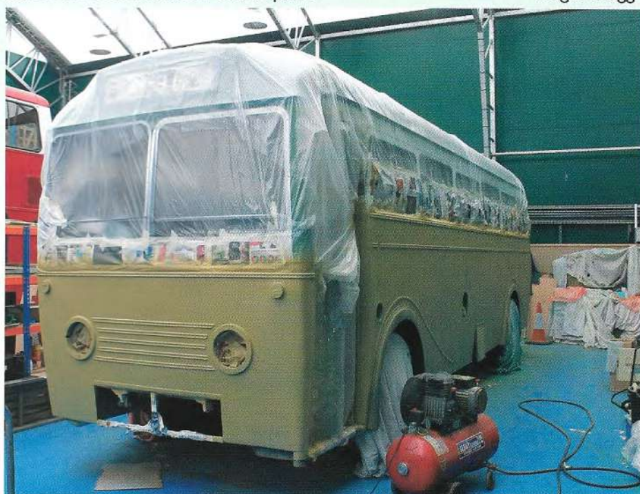
UMP 227 undergoing external repaint.
