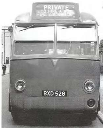
Left: A front view of Q7B reveals the clean lines of the design, with no chassis members visible.
