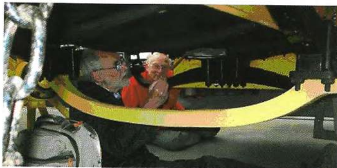
The writer watches while David Pinniger pastes a tissue sheet to the underside of the knifeboard horse bus to check on woodworm activity. (David Williams)
