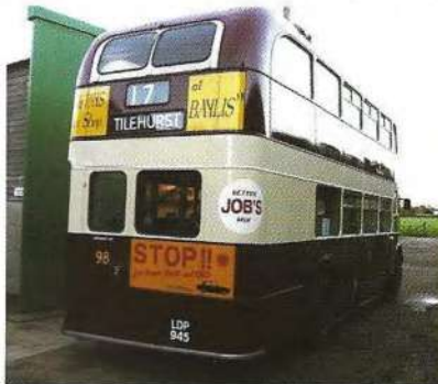
The 1955 ex-Reading Transport AEC Regent III with a Park Royal lowbridge body.
