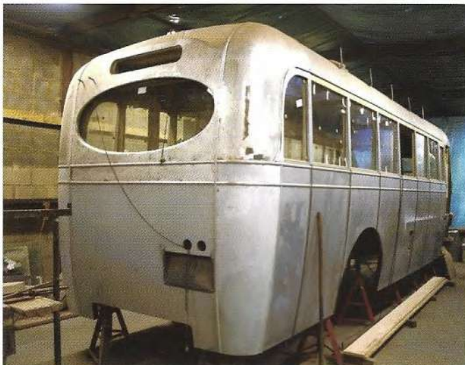
The rear-entrance body of the Leyland Lion had been extensively reframed and repanelled.
