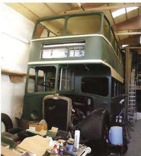
The rear-entrance body of the Leyland Lion had been extensively reframed and repanelled.
