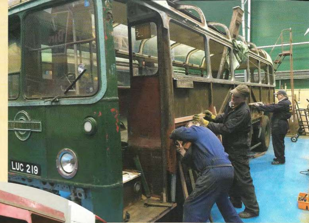
Above: Tin worm and woodworm are eradicated on RF 19.
