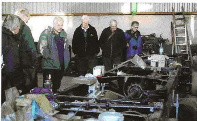
Colin Billington, third from the left, views the Leyland Lion chassis with LBM Members. He described how the frame had needed extensive straightening off-site and indicated parts that had been cast and custom-made in connection with the project.
