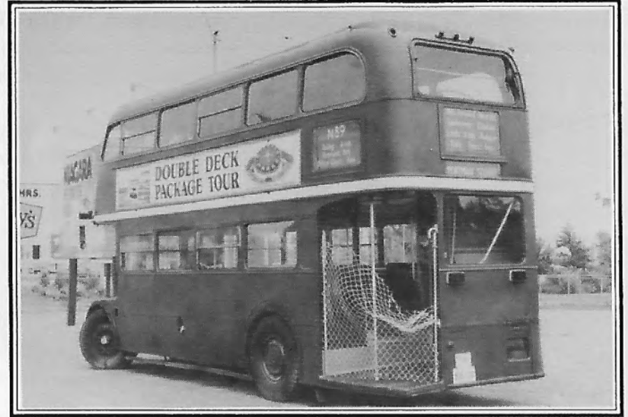
Above. RTL 1315 with the additional marker lights and the rather in-effective rear platform door. Below. RT 3491 with the platform and platform riser removed after major surgery and prior to the transplant.
