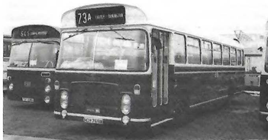
One of more than 100 Bristol REs in preservation, ex-Trent 285 is rare, having the standard ECW bus shell, but with high chassis platform and dual purpose interior; with its Leyland engine, its designation is RELH6L
