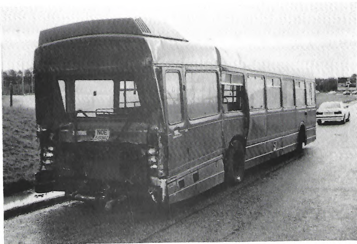
VII) The 'Police Aware' sticker would indicate that it had been dumped, but ex-Midland Red NOE 599R still had a current tax disc and had obviously been hit heavily from behind and pushed into another vehicle, with dramatic consequences. Glad I wasn't at the wheel! (Photo: Mike Nash)
