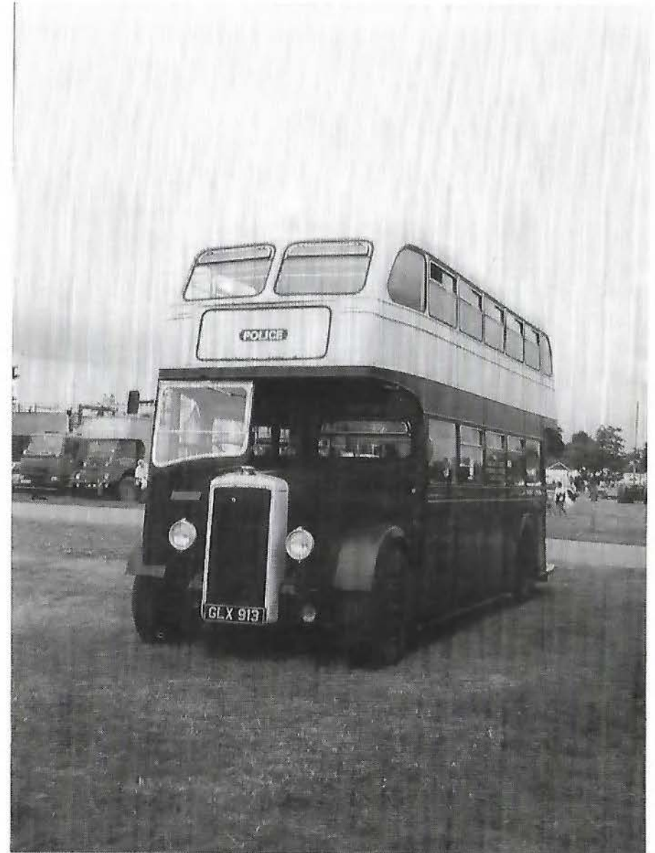
Former D27 suffered the fate of most utility buses when its original body was replaced, in this instance with a Massey body. After service with Southend from 1954, it was used from 1962 carrying a road safety exhibition for Essex police. It is currently preserved in this guise and was seen in July at Ardingley Photo CBM
