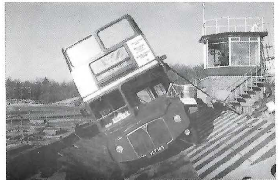
Photo: CBM RM163, the first extra-long RM conversion, being tilt-tested at Chobham as a pre-requisite to certification.
