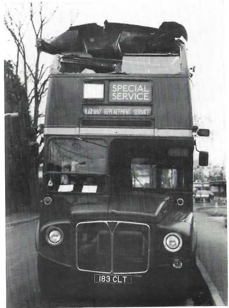
Ouch! The sorry sight of Nostalgiabus RM1183 after it had tried to go under the low bridge at South Ruislip station on 7 December 1997 whilst on Central Line replacement work. Despite its injury, the RM was repaired and back in service within two weeks. Sadly, RM1183 was destroyed in a mindless arson attack on 30 December.
