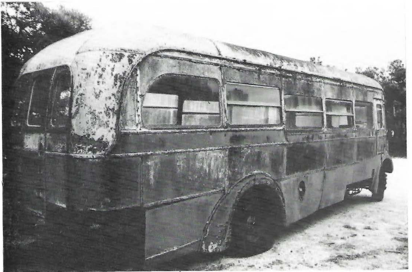
This rear view shows the damage which was probably done when T499 was dragged onto the low loader at the farm. The centre and two corner panels came off as one unit!
