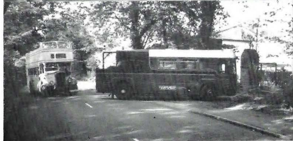
Reporting for Duty... Towbus 332W has been more active this season than for many years. D142 suffered a failed clutch component on its return from the South Coast Run resulting in this busy scene (top) at Dorking, whilst a seized engine on CDL899, one of the Southern Vectis open-toppers, whilst heading to Cobham for August's Display Day saw our tow-bus rescue it from Hindhead. (Photographs: Andy Barnes and Mike Nash).
