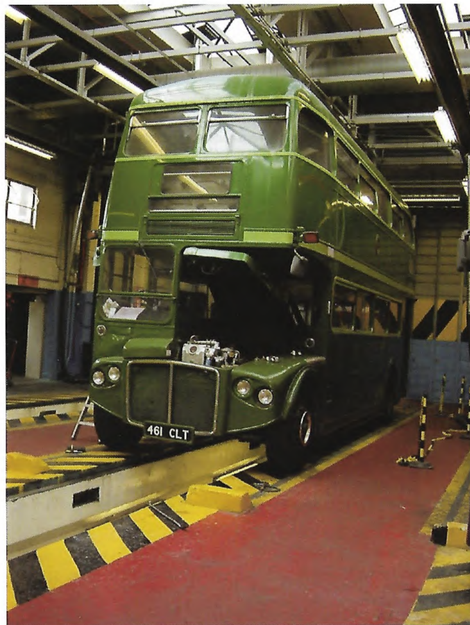
Cobham's new addition RMC1461 over the inspection pit at Romford Garage awaiting an engine change prior to its MOT examination. Photo: Dave Jones
