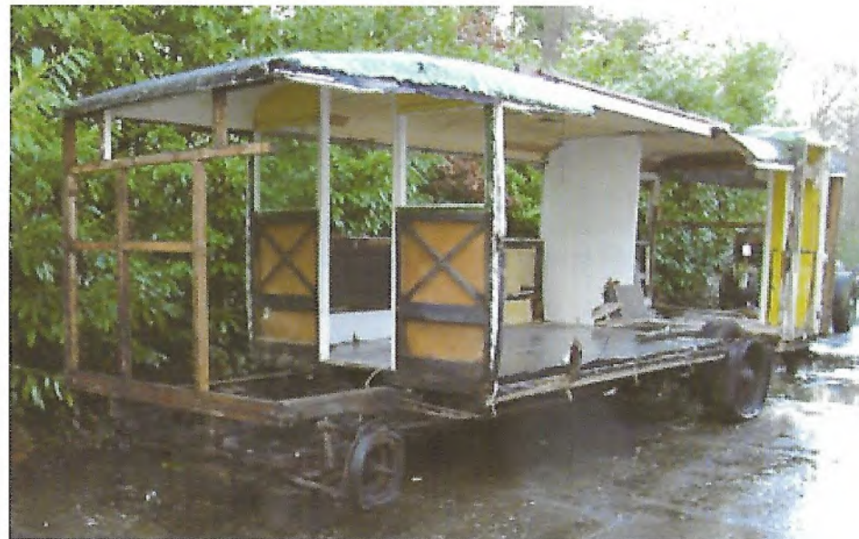
Dennis E Type OT 8902 at Cobham following removal of non-original additions. Front bulkhead is the original.
