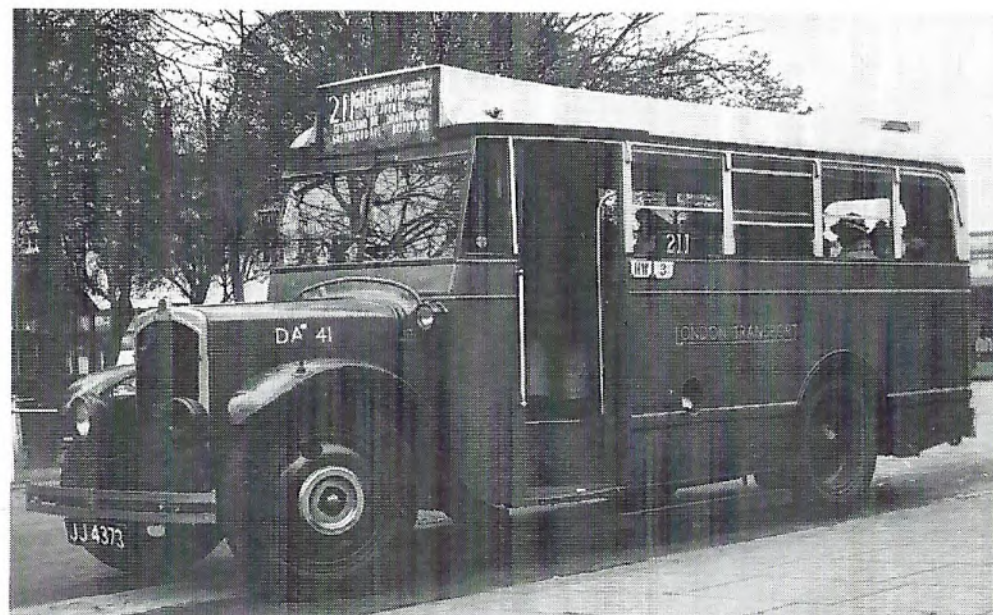
One of the two Dennis Darts specially designed with narrow bodies for working the 211. DA41 at the Ealing Broadway terminus. Photo:J.Higham Copyright:A.Cross
